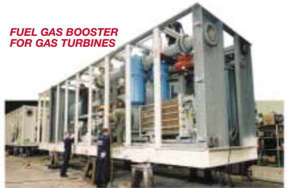
FUEL GAS BOOSTING UNIT FOR 1.8 MW GAS TURBINE LOCATED IN RUSSIA
